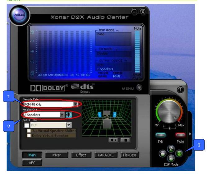
2. Set analog output to 2-speaker mode (to get rid of any channel processing over RMAA stereo signals in the driver) If the Windows platform is Vista, please mind to also select "2 channels" for Audio Channel as the following picture.
