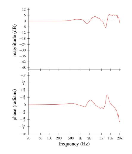
Head-Related Transfer Function (HRTF) measured on Neumann KU100 dummy head at front direction (0 deg azimuth, 0 deg elevation). Source: SADIE II database (York Univ.)
