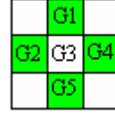
Fig 6. Edge-directional interpolation. G1, G2, G4, G5 – given green pixels, G3 – interpolated green pixel.
