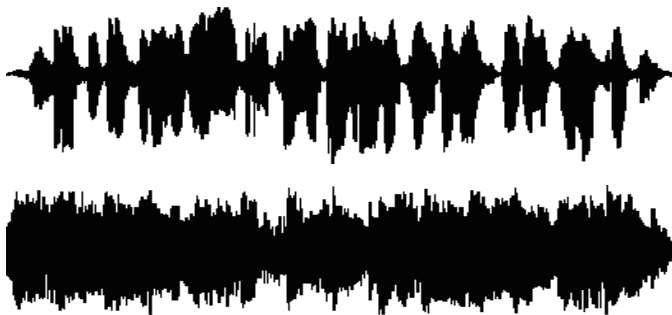
Figure 13: Amplitude envelope of speech (upper) and music (lower). The dynamics of speech is significantly higher.
